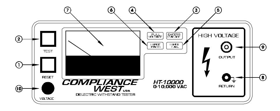
Figure 3-1. Controls, Indicators, Connectors - Model HT-10000 Front Panel
