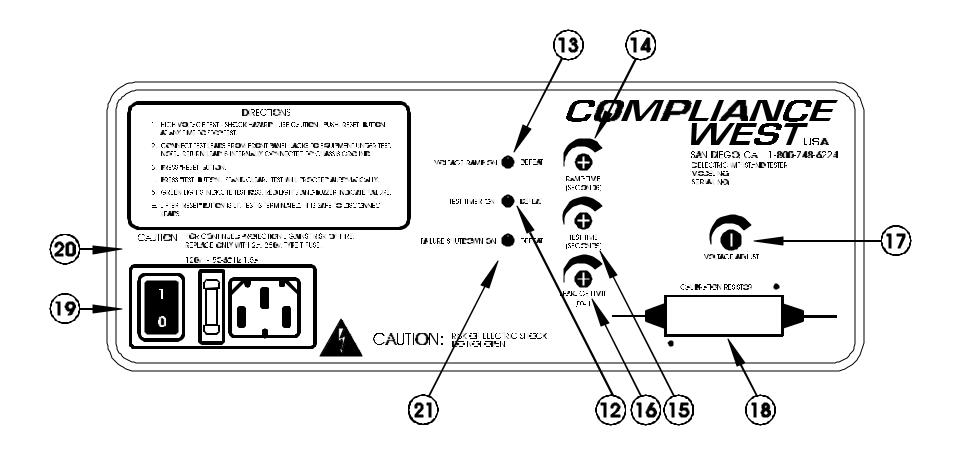
Figure 3-2. Controls, Indicators, Connectors - Model HT-10000 Rear Panel
