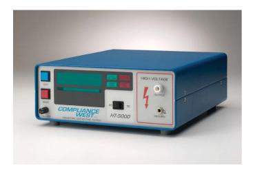
DIELECTRIC WITHSTAND [ HIPOT ] 5000 Vac @ 10mA; 6000Vdc @ 5mA
