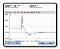
switching, lightning, transformer energization, and load shifting, are immediately characterized as impulsive or oscillatory and detailed for further analysis. Capable of capturing the complete power quality spectrum, the PowerXplorer provides scope-like display of the entire transient.
