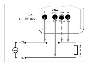
The instrument automatically selects the measuring range which provides maximum resolution for the current measured quantity.
