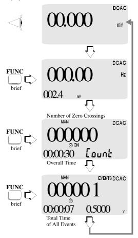
You can switch between two different time displays with the MAN|AUTO key:
