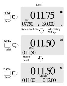
Alternating voltage applied to the jacks appears at the right hand sub-display.
