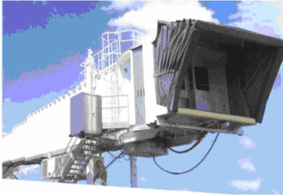
A typical jetway will have a 60-400 Hz solid state or M-G set power converter for “shore power” when it docks
