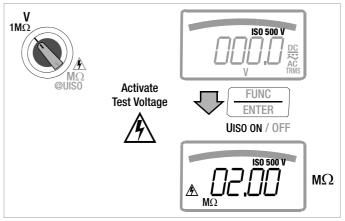
Auto-ranging is active during insulation resistance measurement.
