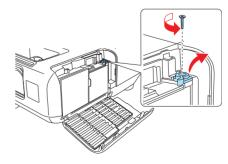
4 Insert the wireless LAN module into the port.
