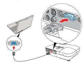
Connect one end to the projector's **Computer (Component Video)** port, and the other end to your computer's | monitor port. If you are using a notebook, switch it to external display. You can also connect an audio cable.
