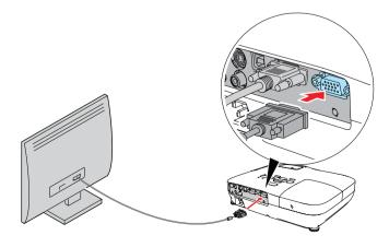
**NOTE:** To use an external monitor, your computer must be connected to the **Computer (Component Video)** port, not the USB port.
