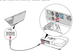
Follow the on-screen instructions to install the Epson USB Display software (only on first connection). Then press the **USB** button on the remote control.
