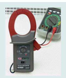
Banana plugs connect into standard multimeter sockets
