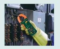
Large jaw size for high current measurements
