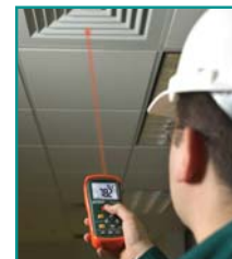
Model AN200 features built-in non-contact IR Thermometer to measure surface temperature that may be hard to reach
