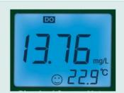
Large blue backlit dual LCD display with calibration and memory indicators
