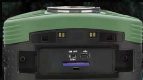
3. Pull off the battery cover by lifting the latch as shown at the right.
