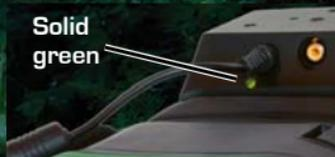
When fully charged, the charging indicator will be lit solid green. The initial charge time is approximately 4 hours.
