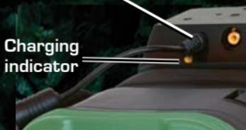
When charging correctly, the charging indicator will be lit yellow and will blink green for one second within about 35 seconds.
