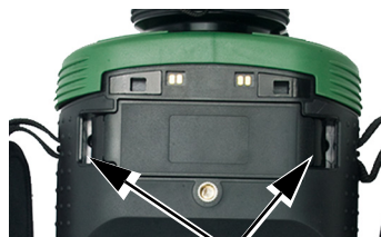
Grasp SD card door edges and pull
