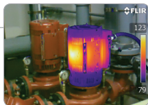
Thermal Fusion inserts IR image set within a temperature interval onto corresponding digital image.
