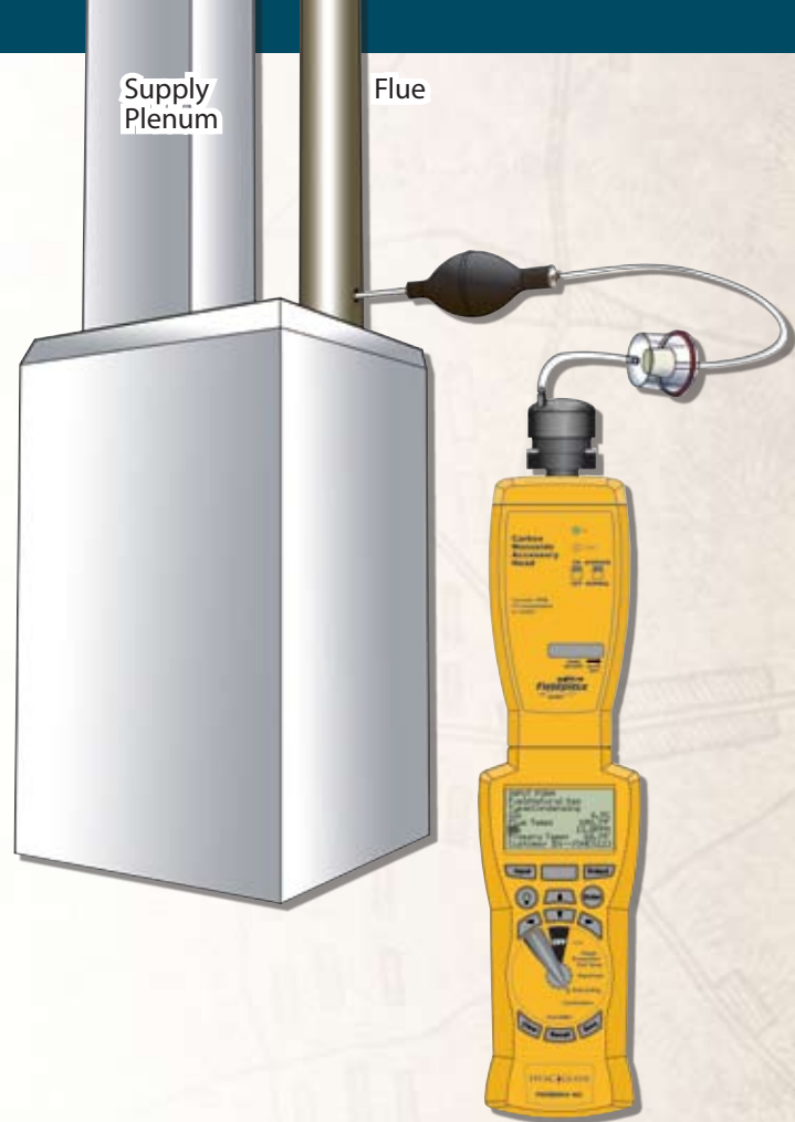
Figure 17. CO measurement of flue gas for the Combustion Test using an ACM3 Carbon Monoxide Head and the AOXP2 pump that's included with the AOXP2 Combustion Check Head.
