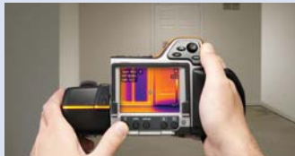
Infrared cameras quickly locate moisture related problems
