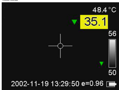
Figure 10.6 A selected color alarm. Press the navigation pad up/down at this stage to increase/decrease the color alarm temperature.
