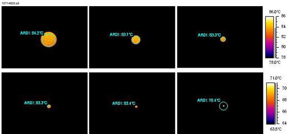
Figure 14.20 Temperature readings from a blackbody at +85°C (+185°F) at increasing distances (24° lens)
