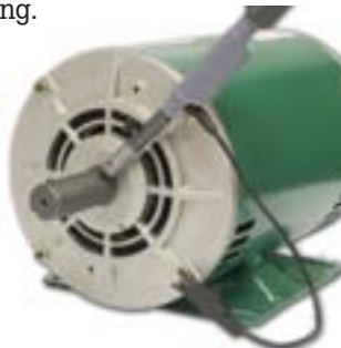
Measuring motor shaft voltage with an Aegis shaft voltage probe (Photo courtesy of Electro Static Technology).
