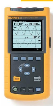
The Fluke 43B Power Quality Analyzer performs the measurements you need to maintain power systems, troubleshoot power problems and diagnose equipment failures. All in a rugged handheld package.
