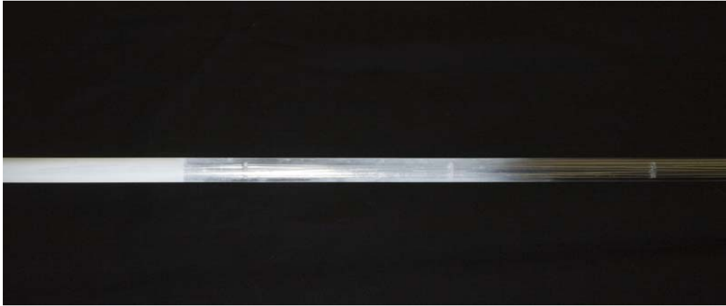
Figure 2: Devitrification of a fused-quartz glass sheath
