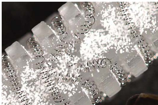
This sensor was damaged by shock during shipping and handling
