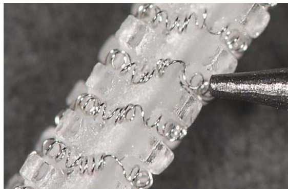
This sensor was damaged by vibration. Notice shorting of coils.
