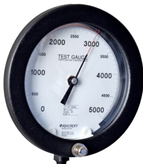
Figure 1. High pressure instruments such as the analog gauge pictured here are often calibrated using hydraulic test media.
