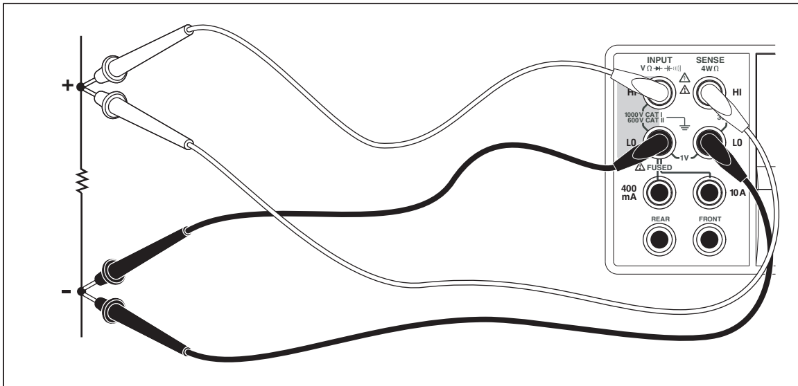
Figure 4-2. Input Connections for 4-wire Resistance Measurements
