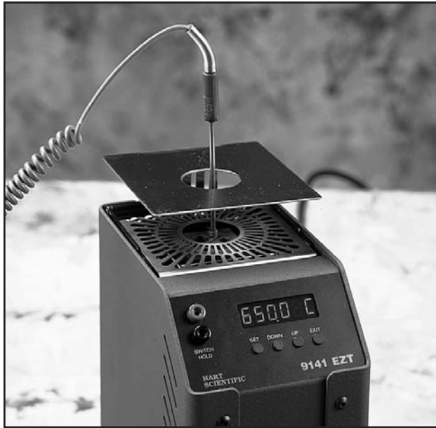
Figure 1 Heat shield installed on 9141 calibrator
