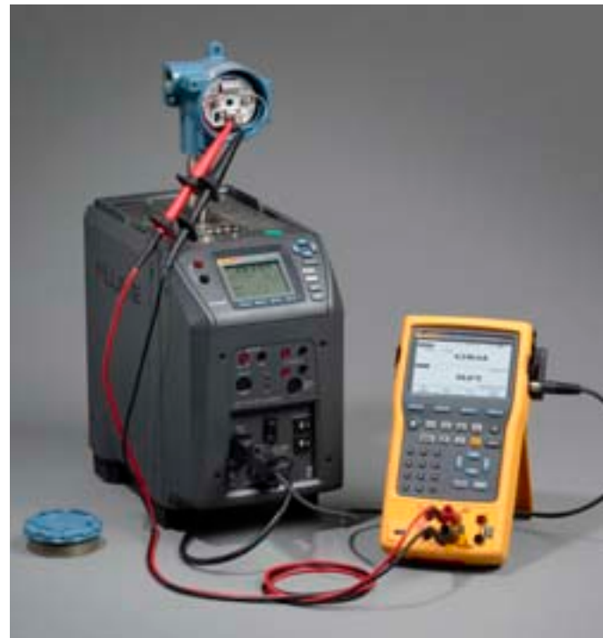
Figure 5. Fluke 754 and Fluke Calibration dry-well calibrating a 4-20 mA transmitter and temperature sensor.
