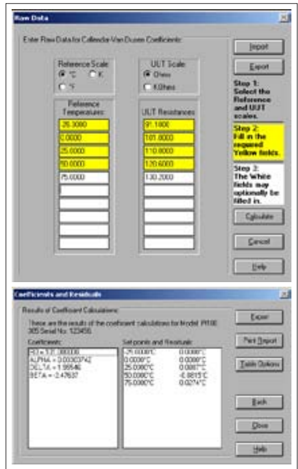
Figure 6. TableWare software from Fluke Calibration calculates unique CVD constants that match the characteristics of the probe.
