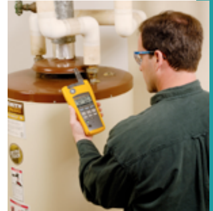
Technician using the 975 AirMeter to check for carbon monoxide leaks.
