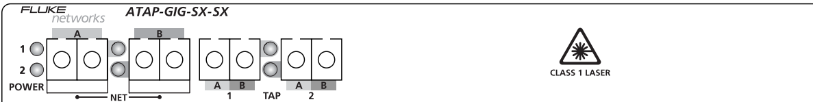
Figure 14. ATAP-GIG-SX-SX Link Aggregating In-Line Tap front panel display
