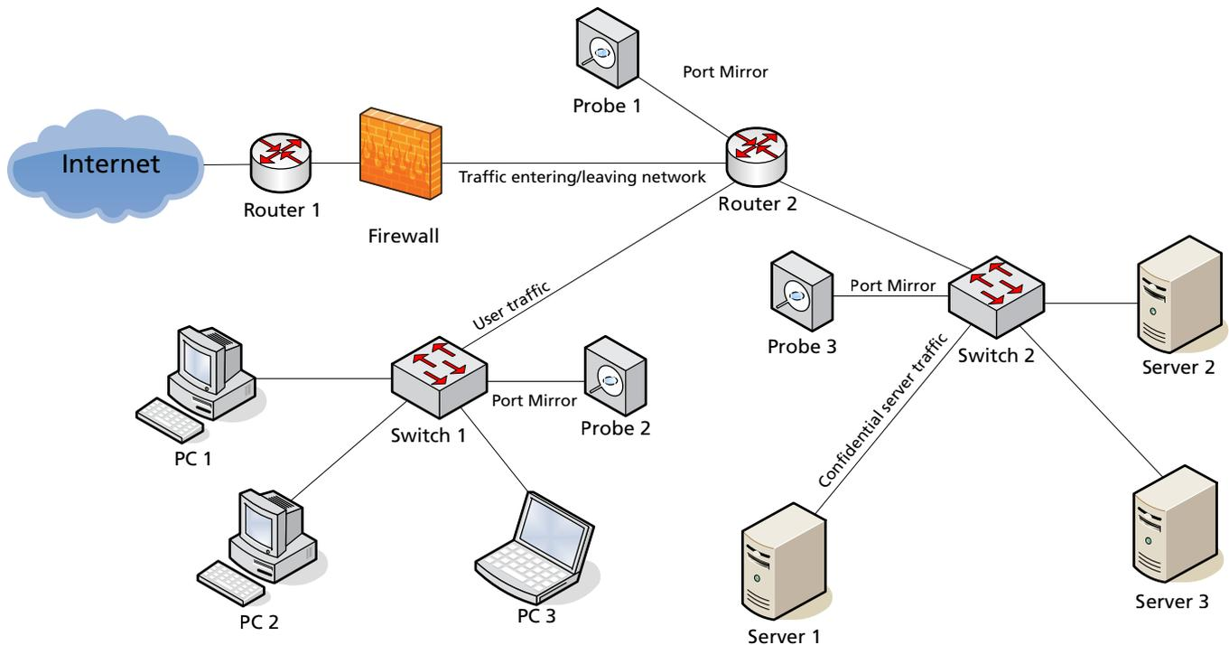
Figure 2: Probe deployment using port mirrors
