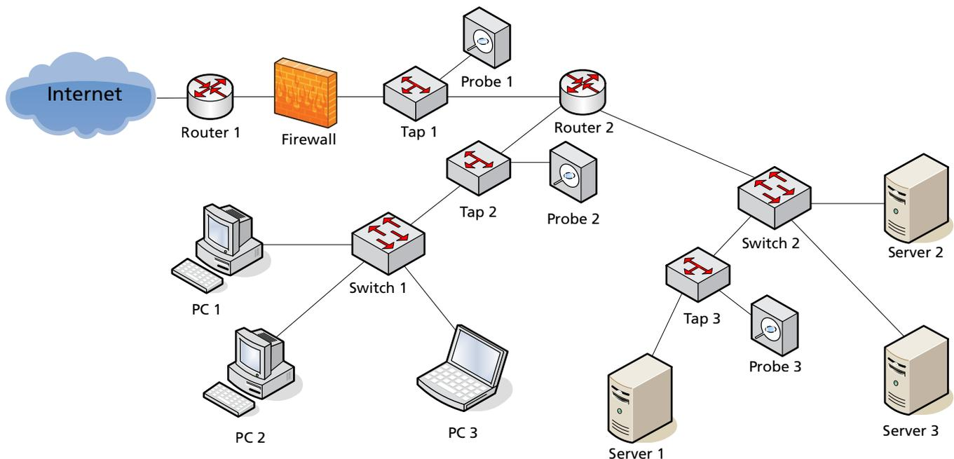
Figure 3: Probe deployment using network TAPs
