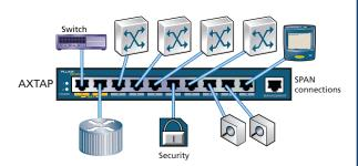
Combination tap replicating and aggregating data from critical router/switch link and 5 SPAN ports to three different analysis solutions.
