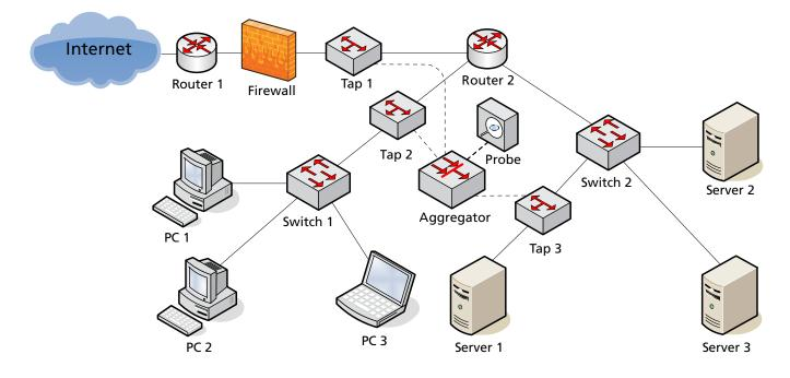
Figure 4: Aggregation of traffic from multiple TAPs to a single Probe
