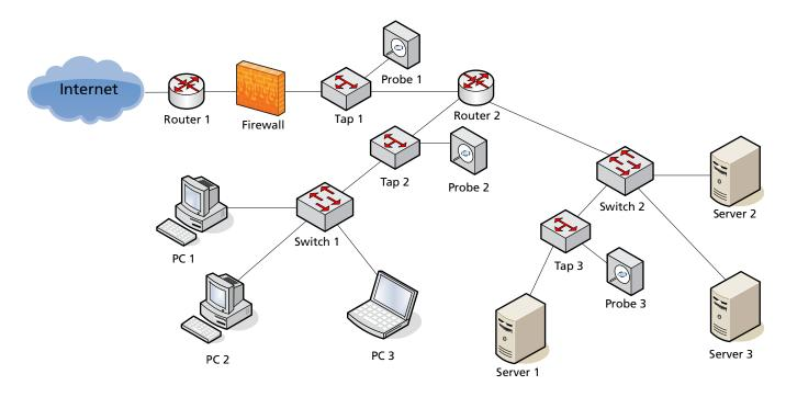
Figure 3: Probe deployment using network TAPs
