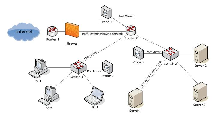
Figure 2: Probe deployment using port mirrors
