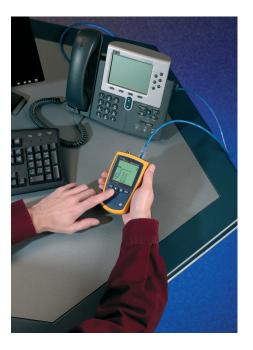
virtually any cable or wire pair, regardless of work environment. Use digital mode to locate high-grade data cabling (Cat 5e/6/6a) in bundles, or at switches, patch panels, or wall outlets. Or, use analog mode on voice-grade cabling (Cat 3 and below), as well as coax, security/alarm, and speaker wiring.
