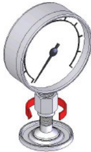
Figure 2-2. Making Pressure Connections
