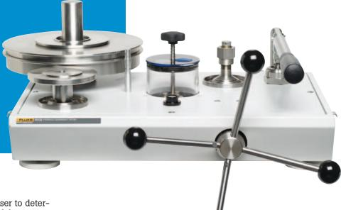
The most accurate method for the user to determine the acceleration of gravity at the laboratory or other site where the deadweight tester will be used is to have a site survey performed. There are various companies that can provide this type of service. Although this is the most accurate method, it can also be expensive.
