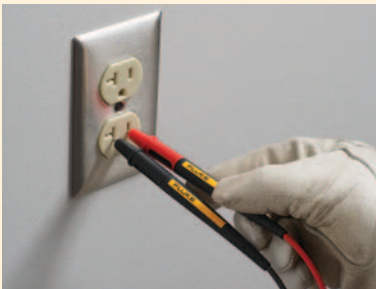
Increase tip exposure for CAT II probing
