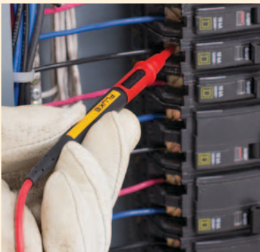
Reduce tip exposure for CAT III testing
