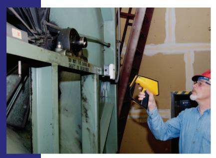
Many facilities monitor this type of equipment on a regular basis, because often a simple problem like lubrication can be spotted and fixed inexpensively, before the entire unit burns out. Such strategies fall under the general heading of predictive maintenance (PdM).
