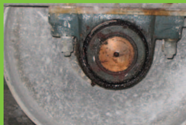
This overheating shaft and bearing may be an indicator of bearing failure, lack of proper lubrication, or misalignment.
