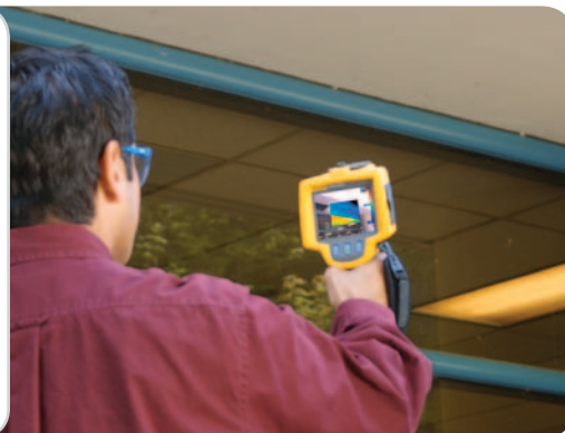
Roofing: Detect water-saturated insulation in flat-roof systems to locate damaged portions of roofing structure.
