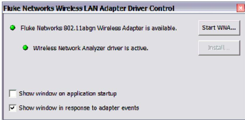
The green radio button next to the **Wireless Network Analyzer driver is active** field indicates that the Wireless Network Analyzer application is using the drivers. You can disable the **Show window on application startup** and **Show window in response to adapter events** checkboxes if you do not wish to see the popup. Press the **Start WNA** button to begin the application.
