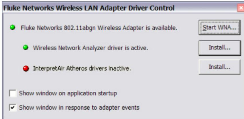
If the radio button next to the application that you want to run is not green, press the **Install** button to make the drivers active. It is recommended that you leave the **Show window on application startup** and **Show window in response to adapter events** checkboxes enabled. If you disable the checkboxes and wish to switch applications, you can select the icon in the system tray to display the Driver Control window.
