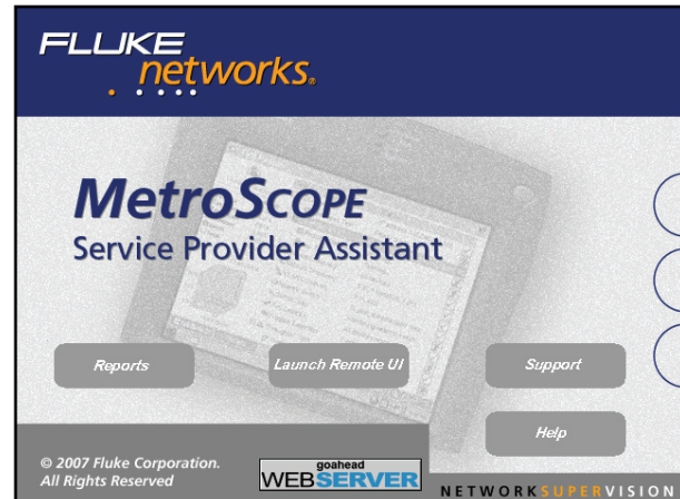
Figure 7: MetroScope's web interface home page provides access to reports, remote control and online help.
