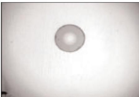
Figure 4: Good/clean fiber endface
