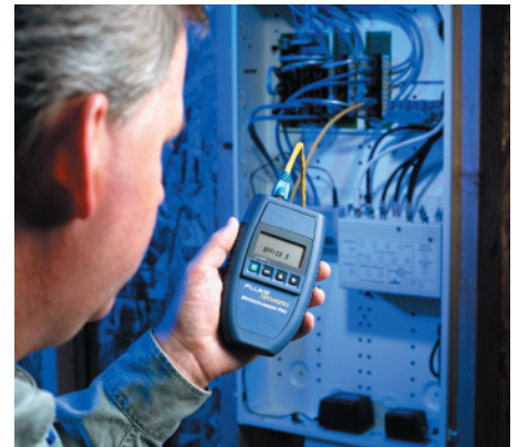
Verification tools are simple, low-cost devices that check the basic connectivity of the installed links.
