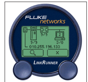
Ping DNS server or key devices, and observe response time.
