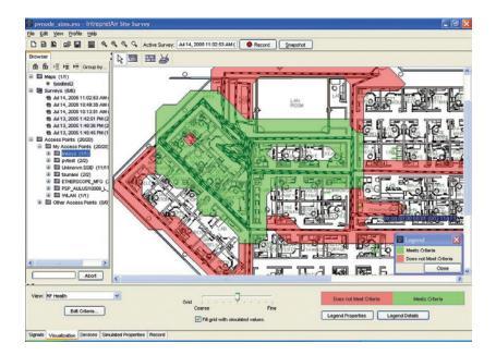
Compared to other site survey products, InterpretAir software, with its unique RF Health feature, takes wireless analysis to a new level by enabling visualization of multiple measurement criteria in a single view, simplifying analysis and accelerating decision making.
