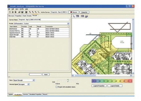
SnapShot, a feature unique to InterpretAir software, accelerates troubleshooting by quickly comparing RF performance at a fixed location against customer defined criteria. Prove the problem is not with the RF physical layer as a first step in troubleshooting the network.
