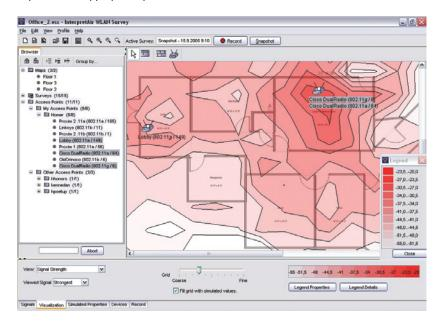
The signal strength visualization indicates areas within the building where additional access points should be installed to ensure persistent connectivity and seamless roaming. Verify wireless performance post installation, and make adjustments to optimize performance.
