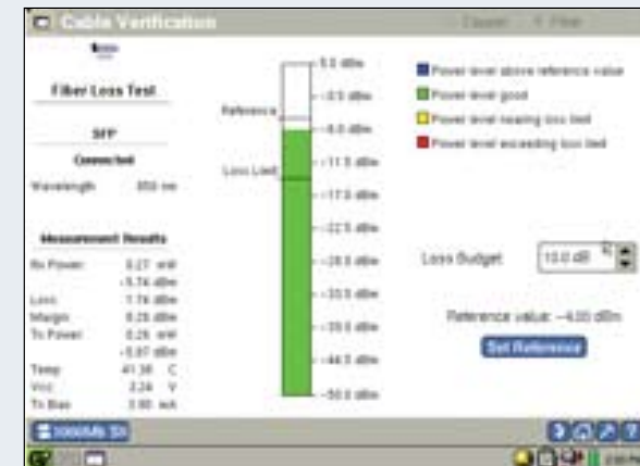
Ensure optical power limits are within specification
