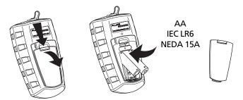
Note: Fluke Networks recommends alkaline batteries.
