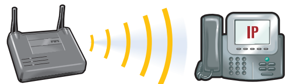
Figure 16: RF interference can reduce the range of VoWLAN phones resulting in unacceptable voice quality or lost of service.
