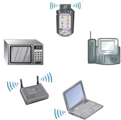
Figure 11: Examples of common items that cause RF interference. You will be amazed at all the items that cause interference.
