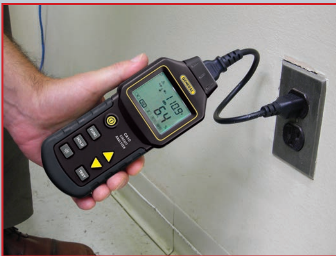
The short test cable improves voltage-drop measurement accuracy
