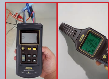
Tracing a cable behind a wall
