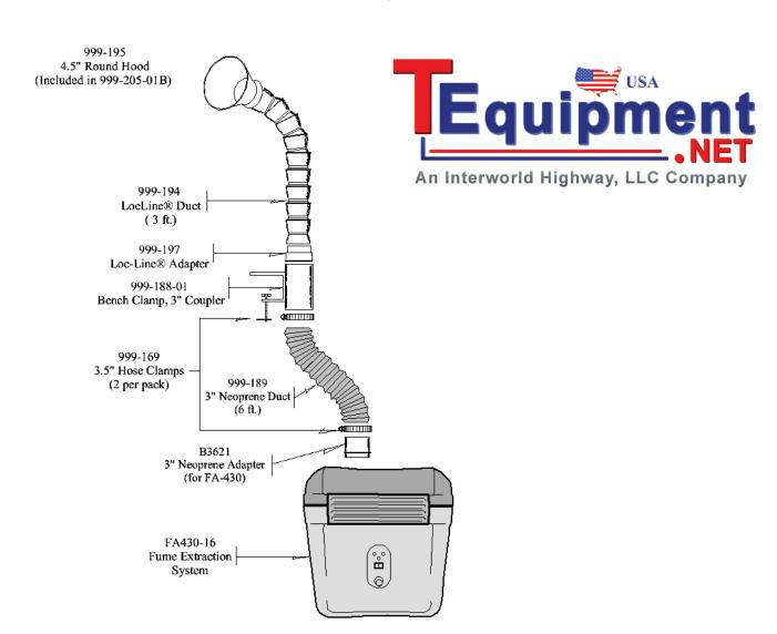
NOTE: Ensure the Neoprene Duct is attached to the longer side of the Neoprene Duct Adapter as measured from the flange.
